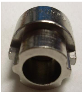
Seal case Socket Tool, 1/2" (DH88596)
