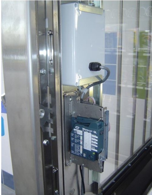
Microcoin QL and Logic PCB
